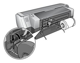
8. Load the paper part of the way into the roll paper feeder (under the white rollers), then slide the right roll paper edge guide to fit lightly against the paper.
